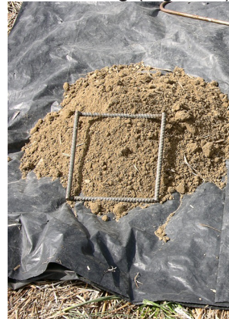
Figure 2. Compact method: 8 inch square by 6 inch deep sample.
