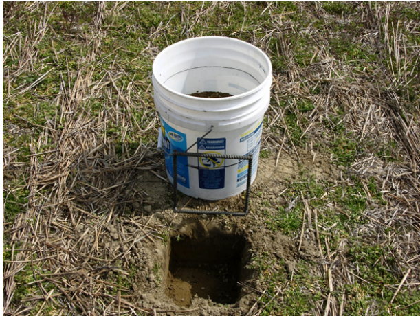
Figure 2. Compact method: 8 inch square by 6 inch deep sample.
